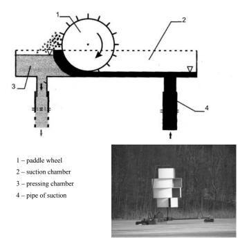
Fig. 2. The scheme of the pulverizer operation [after 21, changed] and photography of the pulverising aerator with vertical Savonius turbine on Lake Góreckie.
